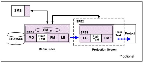
Figure 12: Media Block Server Configuration<sup>10</sup>
