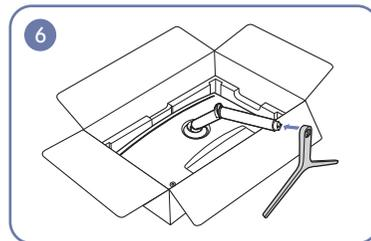
Attach the stand base to the neck, as shown in the image. Make sure there is no gap between the stand neck and base.
