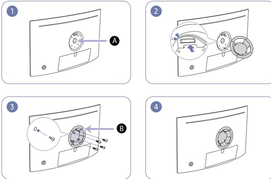
**A** Attach the BRACKET WALL here
