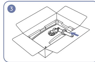
Attaching the COVER-REAR TOP to the stand neck, as shown in the figure.
