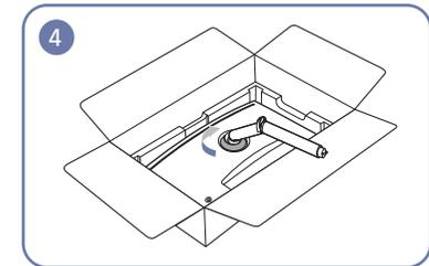
Turn the COVER-REAR TOP clockwise to attach it to the rear cover.
