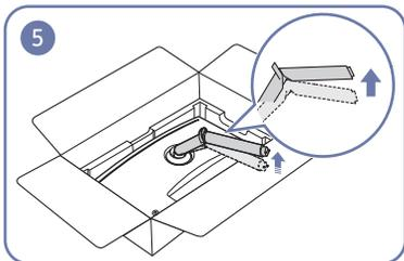
While pressing down with one hand on the lower styrofoam layer, lift the stand's neck with the other hand.
