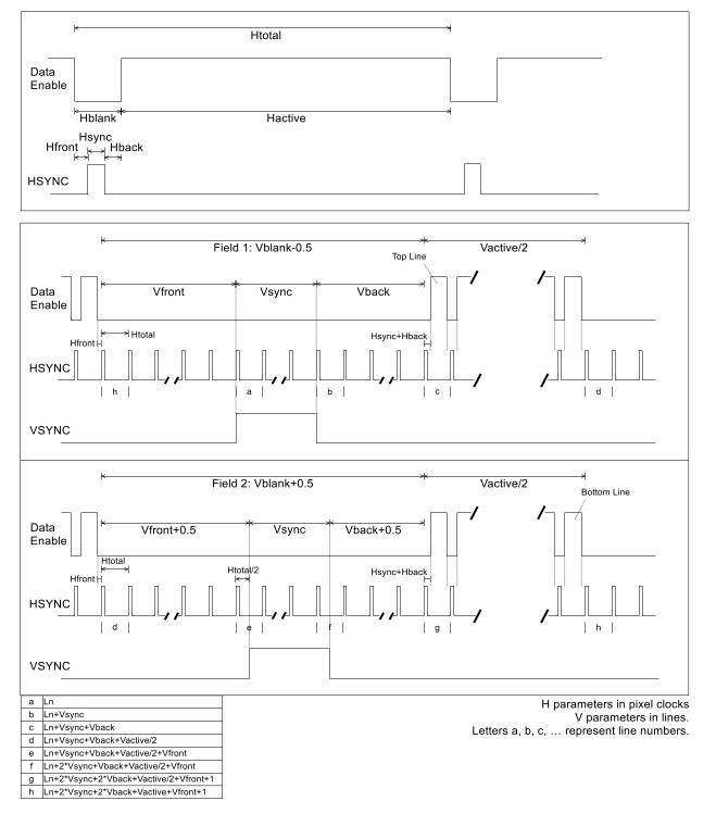
Figure 4. General Interlaced Video Format Timing (Positive Sync)
