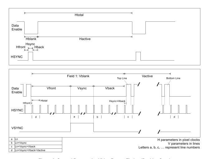
Figure 2. General Progressive Video Format Timing (Positive Sync)
