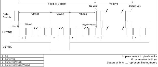
Figure 1. General Progressive Video Format Timing (Negative Sync)
