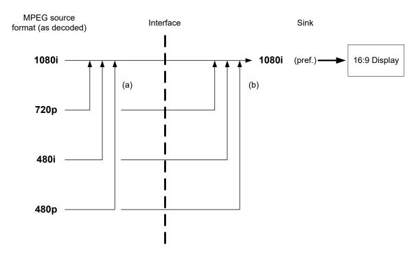
Figure 10 Example of Options for Format Conversion
