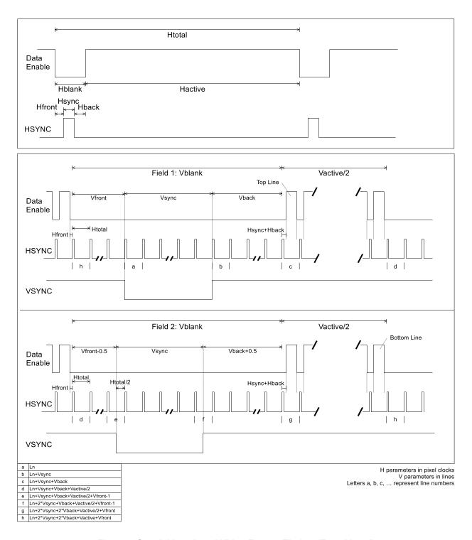
Figure 5 Special Interlaced Video Format Timing (Even Vtotal)
