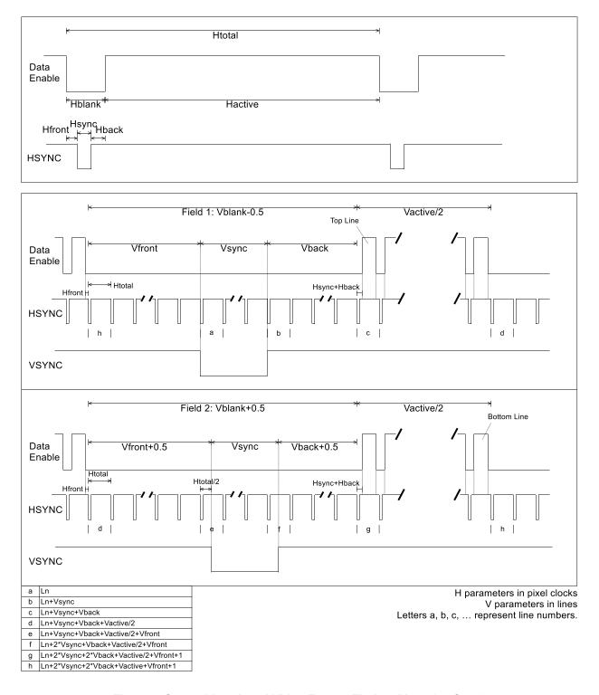
Figure 3 General Interlaced Video Format Timing (Negative Sync)
