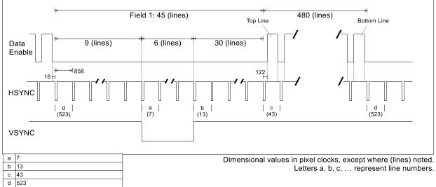
Figure 14 General Progressive Example for Video ID Codes 2 & 3 (720x480p @ 60 Hz)
