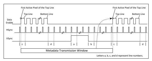
Figure 7 HDR Dynamic Metadata Transmission Window and Metadata Applicability
