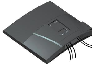
Step 6: Attach the mounting bracket from the VESA compatible wall mounting kit (100mm x100mm distance), the type of VESA mounting screw is M4 x 10 mm.
