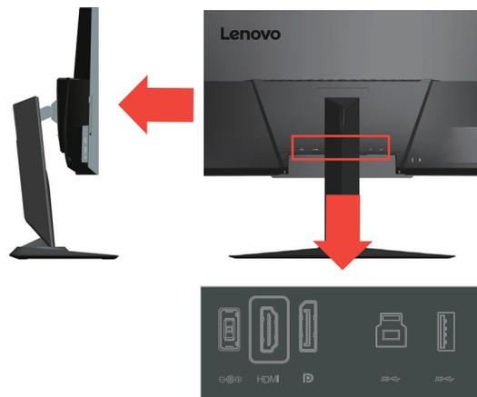
3. Connect one end of the DP cable to the DP connector on the back of the computer, and the other end to the DP connector on the monitor. Lenovo recommends that customers who require to use the Display Port input on their monitor purchase the "Lenovo Display Port to Display Port cable 0A36537".
