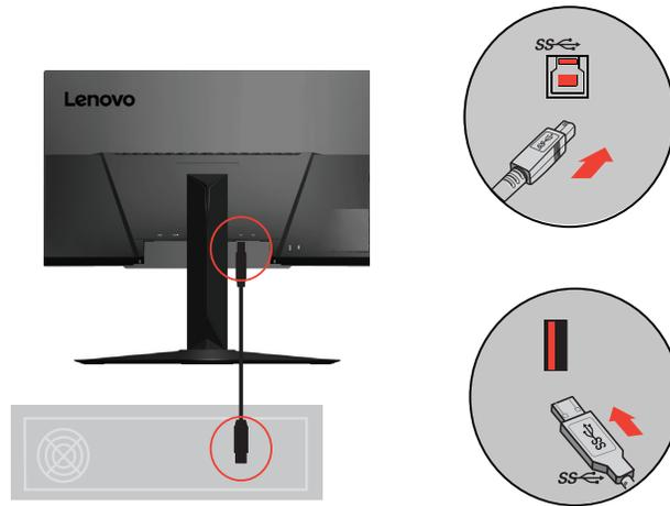
8. Connect one end of the USB cable to the USB downstream terminal on the side of the monitor, and connect the other end of the USB cable to an appropriate USB port on your device.
