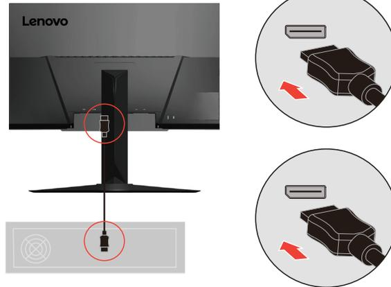
4. Connect one end of the HDMI cable to the HDMI connector on the back of the computer, and the other end to the HDMI connector on the monitor. Lenovo recommends that customers who require to use the HDMI input on their monitor purchase the “Lenovo HDMI to HDMI cable OB47070”.
