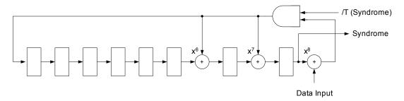
Figure 5-5 Error Correction Code generator
