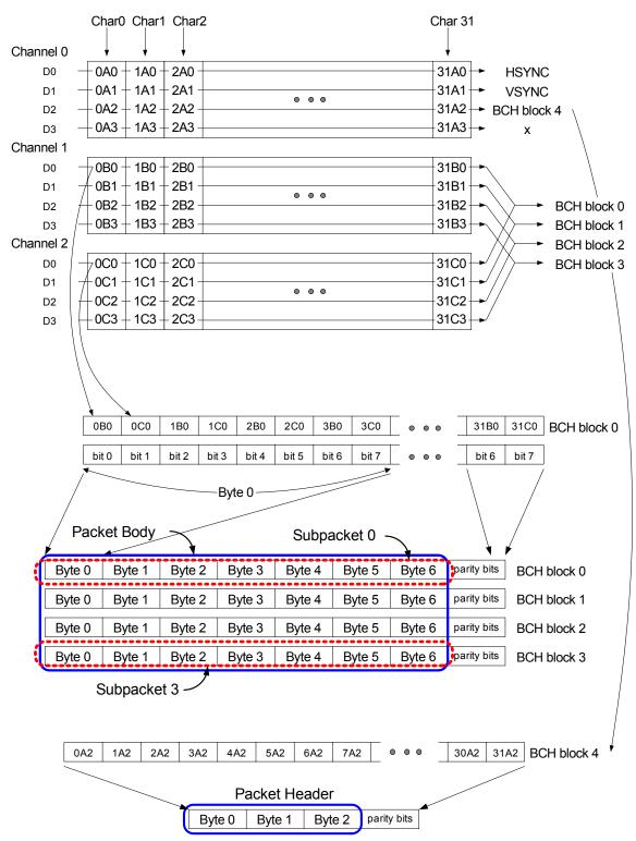
Figure 5-4 Data Island Packet and ECC Structure
