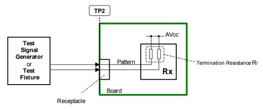
Figure 4-19 HDMI Sink Test Points
