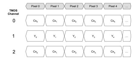
Figure 6-3 8-bit YC<sub>B</sub>C<sub>R</sub> 4:4:4 mapping
