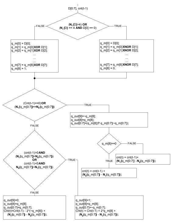
Figure 5-7 TMDS Video Data Encode Algorithm
