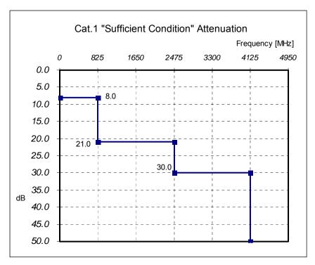
Figure 4-22 Category 1 Cable Attenuation Limits – Sufficient Condition
