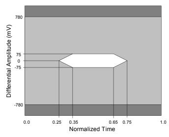
Figure 4-20 Eye Diagram Mask at TP2 for Sink Requirements
