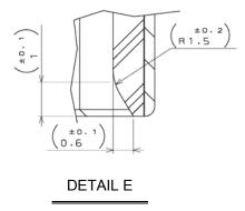
The form shown above is required. This feature will reduce the likelihood of damage to the receptacle insulator under rough operation.
