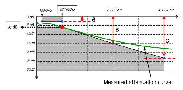
Figure G-1 Passive equalizer Cable Attenuation Limits – Sufficient Condition
