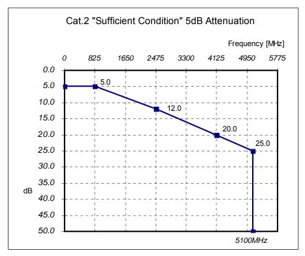
Figure 4-23 Category 2 Cable Attenuation Limits - Sufficient Condition
