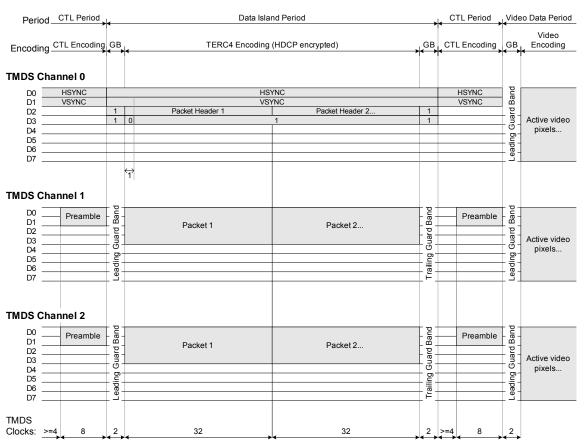
Figure 5-3 TMDS Periods and Encoding
