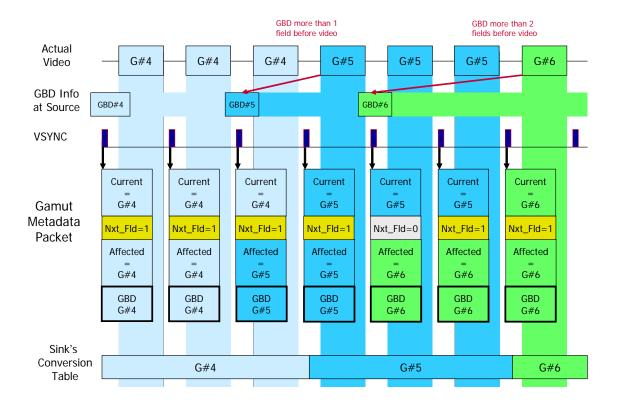
Figure 5-6 Example P0 Transmission Sequence
