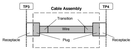
Figure 4-21 Cable Assembly Test Points
