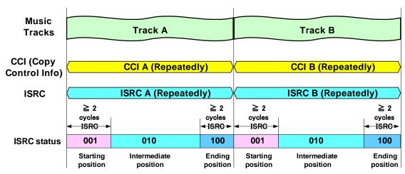
Figure 8-4 ISRC/CCI and ISRC Status Handling
