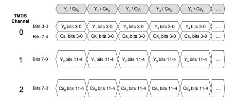
Figure 6-2 YC<sub>B</sub>C<sub>R</sub> 4:2:2 component
