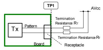
Figure 4-17 Balanced Source Test Load
