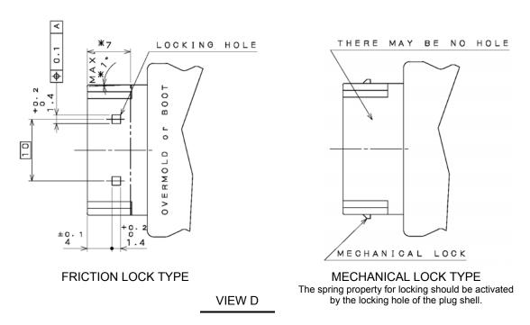
Figure 4-6 Type B Plug Mating Interface Dimensions
