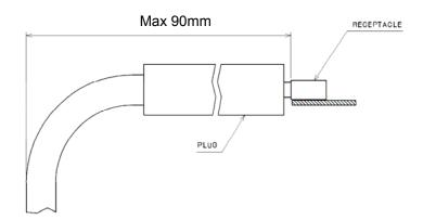
Figure 4-4 Type A Cable – Minimum Recommended Cable Bend
