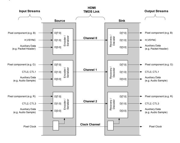
Figure 5-1 HDMI Encoder/Decoder Overview
