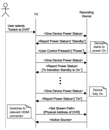
CEC Figure 20 A typical scenario for to discover the power status of a target device
