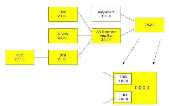
Figure 8-3 Addresses within an HDMI cluster
