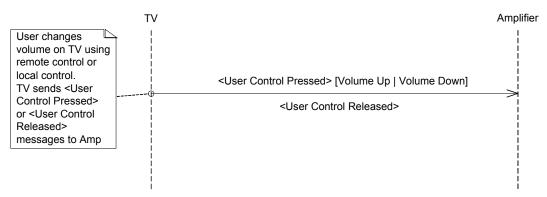
CEC Figure 23 Typical Operation of the volume control
