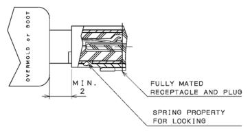
Figure 4-3 Type A Receptacle and Plug Mated Condition
