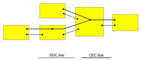
Figure 8-1 CEC and DDC line connections
