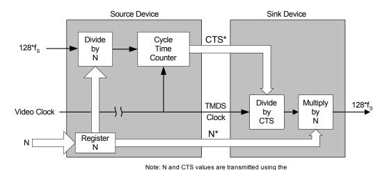
"Audio Clock Regeneration" Packet. Video Clock is transmitted on TMDS Clock Chanel.
