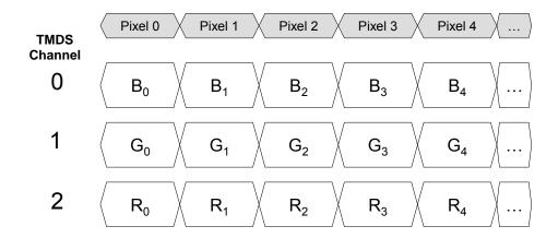
Figure 6-1 Default pixel encoding: RGB 4:4:4, 8 bits/component
