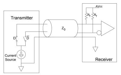
Figure 4-12 Conceptual Schematic for one TMDS differential pair
