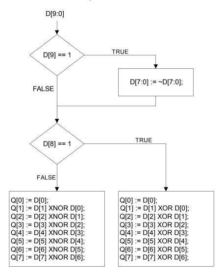
Figure 5-8 TMDS Video Decode Algorithm
