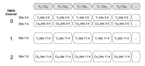
Figure 6-4 YC<sub>B</sub>C<sub>R</sub> 4:2:2 with Pixel-Doubling
