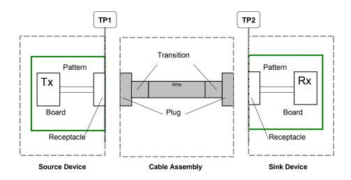
Figure 4-15 TMDS Link Test Points
