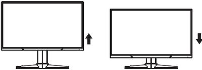
3. Vertical direction can be adjusted up and down within 65mm.
