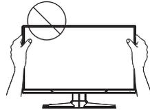
4. When adjusting the angle of the display, be sure not to touch or press the screen area.
