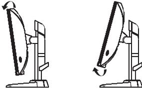
1. The screen may be inclined  $5^{\circ}$  forward and  $20^{\circ}$  backward.
