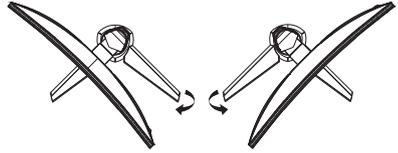
2. The angle may be adjusted left and right within  $-30^{\circ}$ - $30^{\circ}$ .
