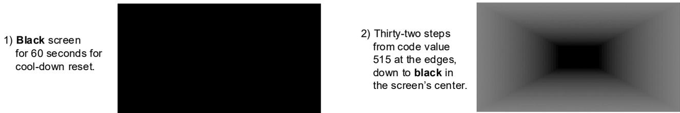
**Figure 5-5: Tunnel Test – Black-level Test Sequence**
