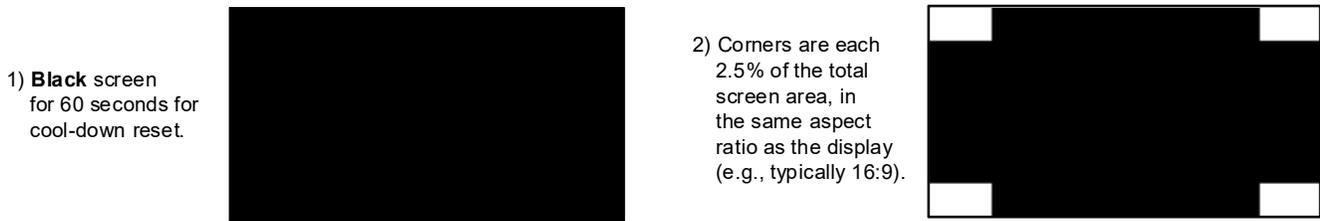
**Figure 5-4: Corner Box Test – Black-level Test Sequence**
