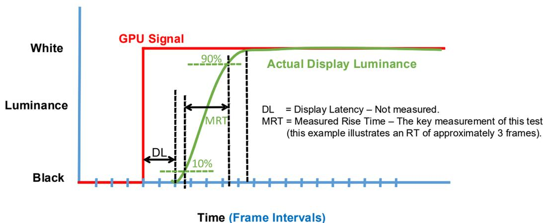
Figure 8-2: Measured Rise-time Illustration
