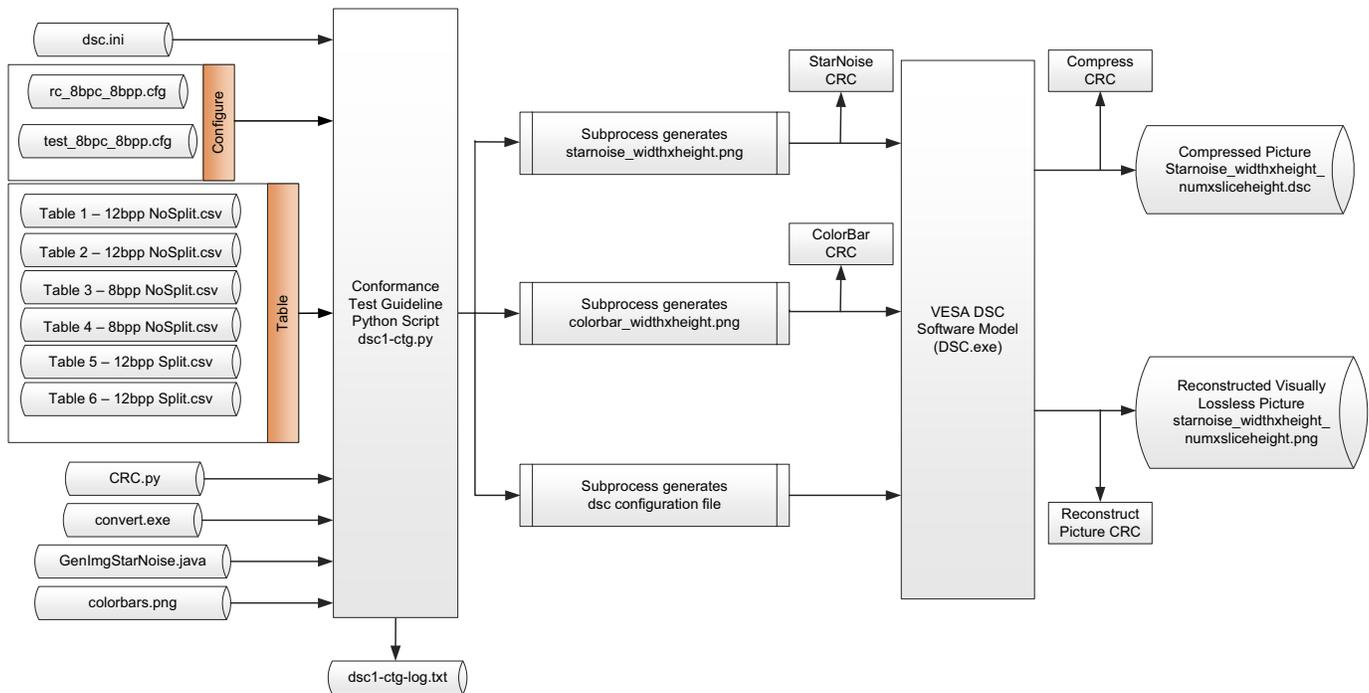
Figure 5-1: Detailed DSC CTG Buffer Conformance Process Diagram
