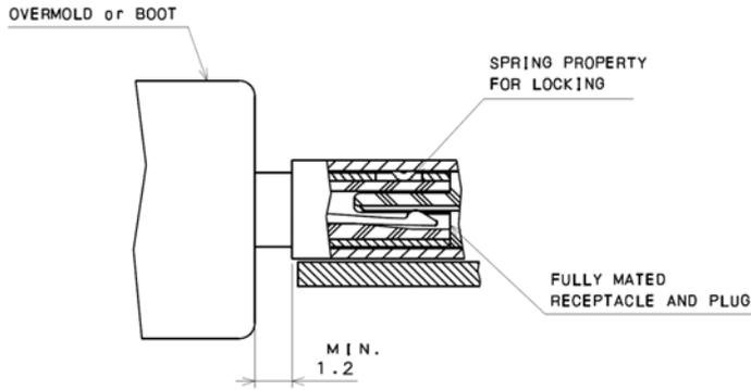
Figure 4-10 Type C Receptacle and Plug Mated Condition
