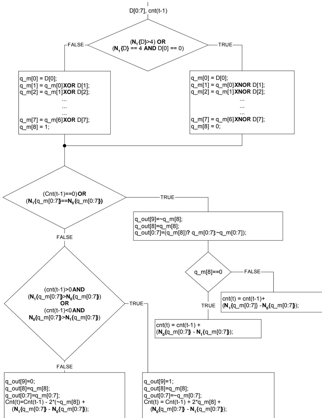
Figure 5-7 TMDS Video Data Encode Algorithm
