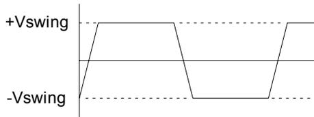
Figure 4-14 Differential Signal
