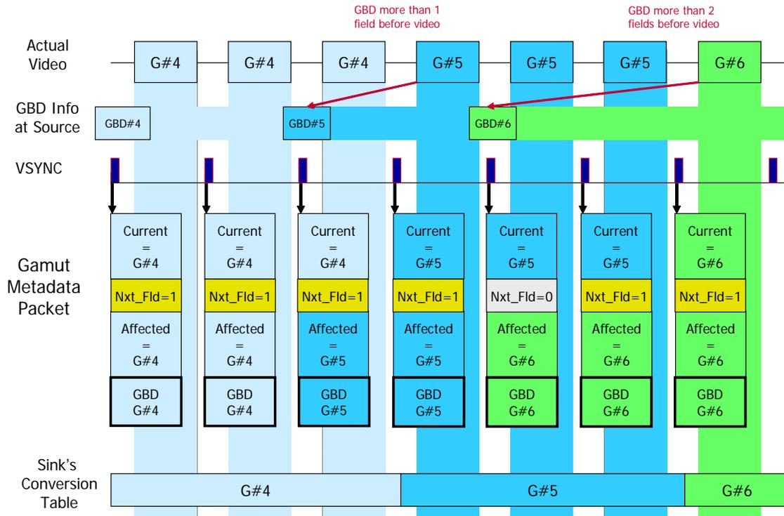
Figure 5-6 Example P0 Transmission Sequence
