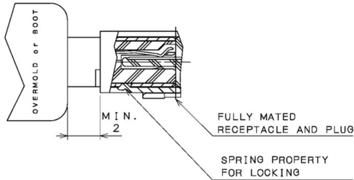
Figure 4-3 Type A Receptacle and Plug Mated Condition
