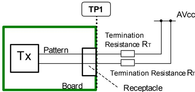
Figure 4-17 Balanced Source Test Load
