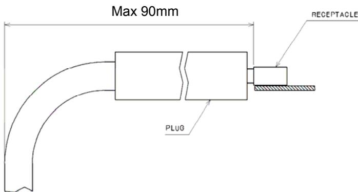
Figure 4-4 Type A Cable – Minimum Recommended Cable Bend
