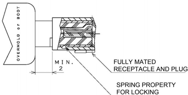
Figure 4-7 Type B Receptacle and Plug Mated Condition
