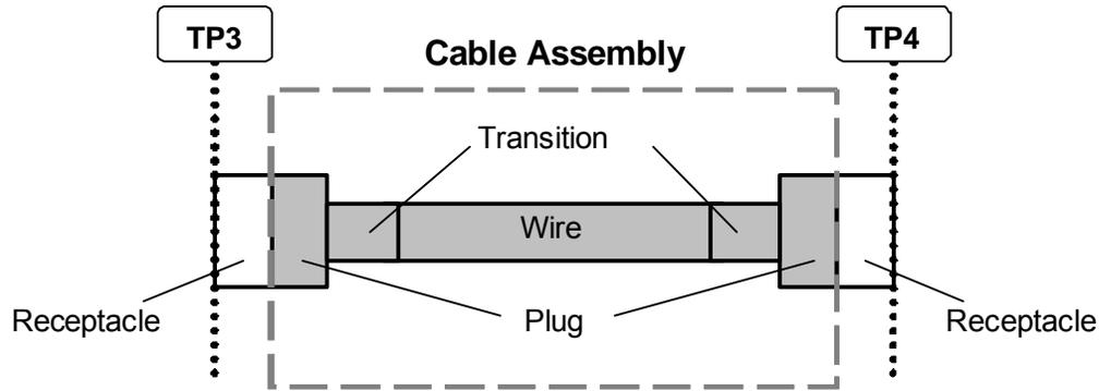
Figure 4-21 Cable Assembly Test Points
