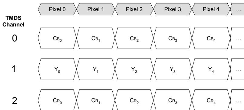
Figure 6-3 8-bit  $Y_C B_C R$  4:4:4 mapping
