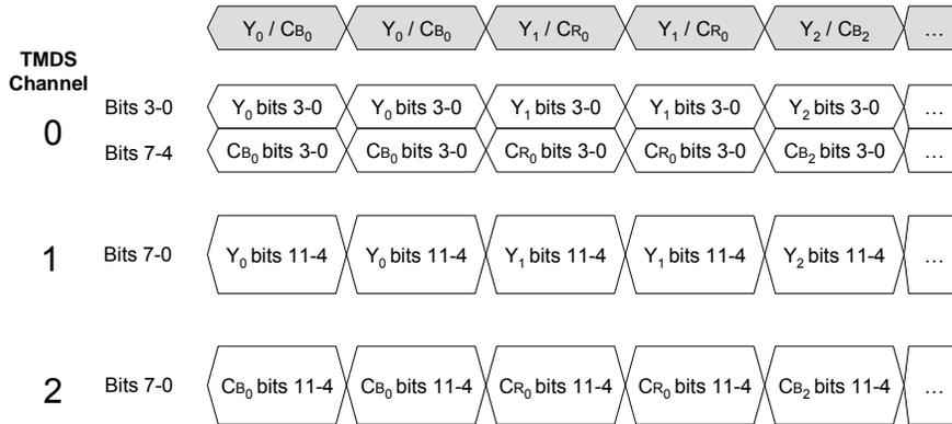
Figure 6-4 YC<sub>B</sub>C<sub>R</sub> 4:2:2 with Pixel-Doubling
