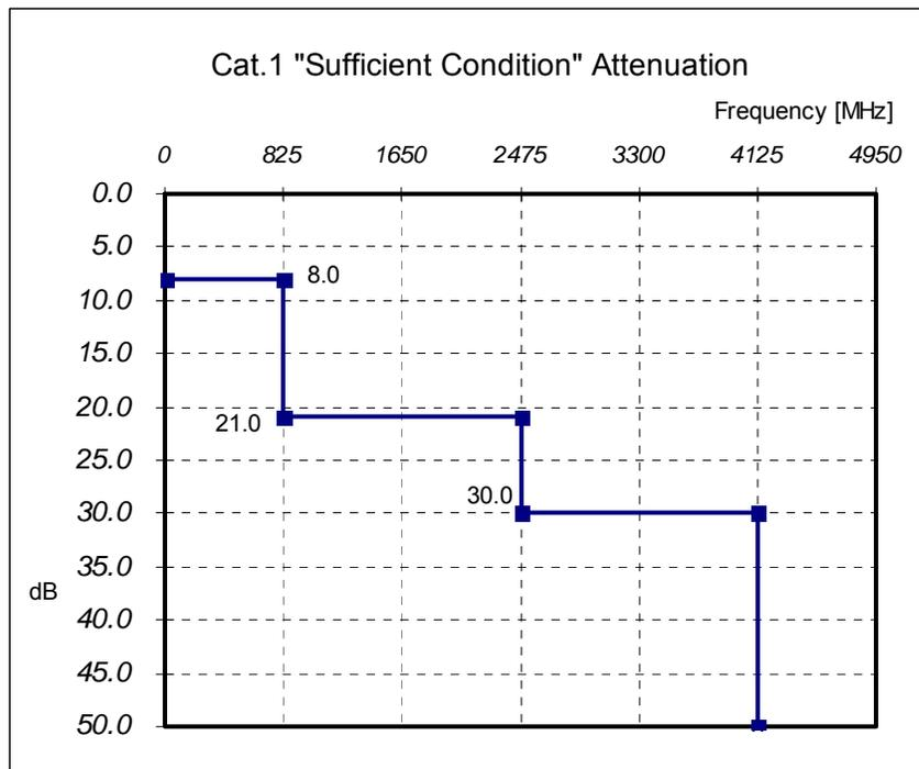
Figure 4-22 Category 1 Cable Attenuation Limits – Sufficient Condition
