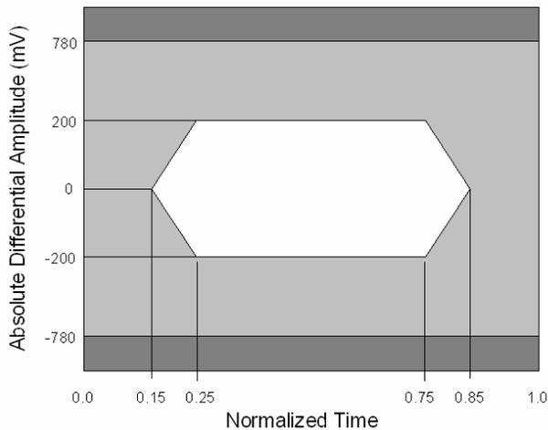
Figure 7-1 Source (TP1) Eye Diagram
