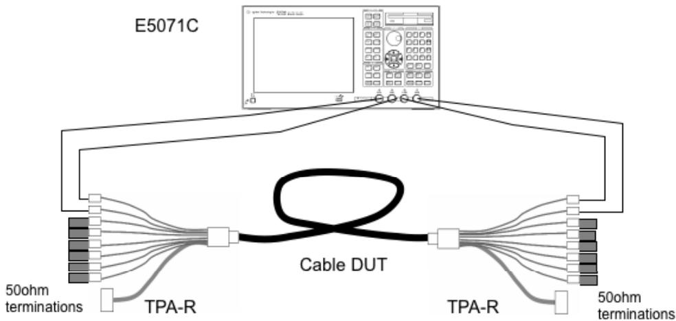
Setup 9. Test ID 5-7: Attenuation and Phase: Agilent
