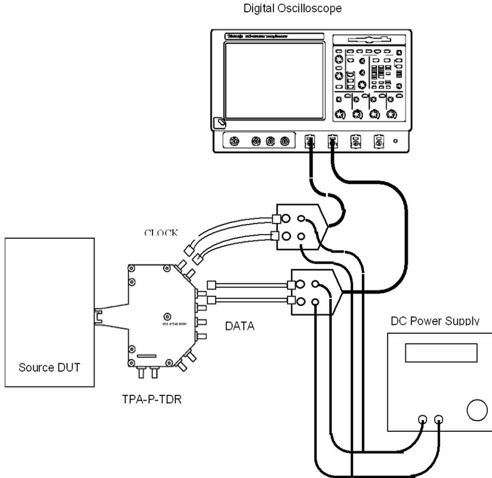
Setup 31. Test ID 7-10: TMDs – Data Eye Diagram - Tektronix TDS7404
