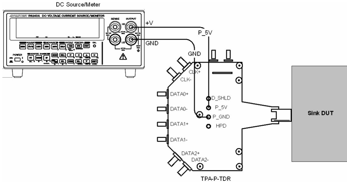
Setup 49. Test ID 8-12: +5V Power Max Current
