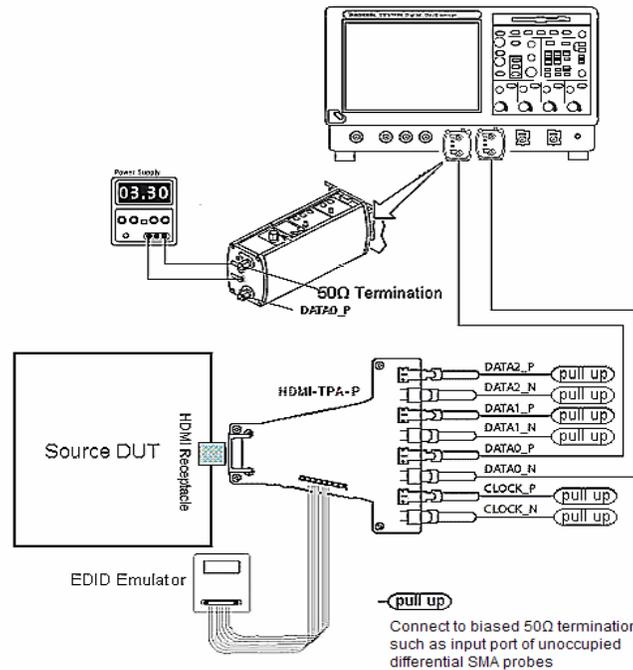
Setup 13. Test ID 7-2: TMDS –VBL: Tektronix DPO70804
