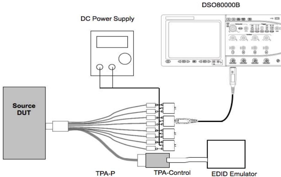
Setup 18. Test ID 7-2: TMDS –VBL: Agilent DSO8000B
