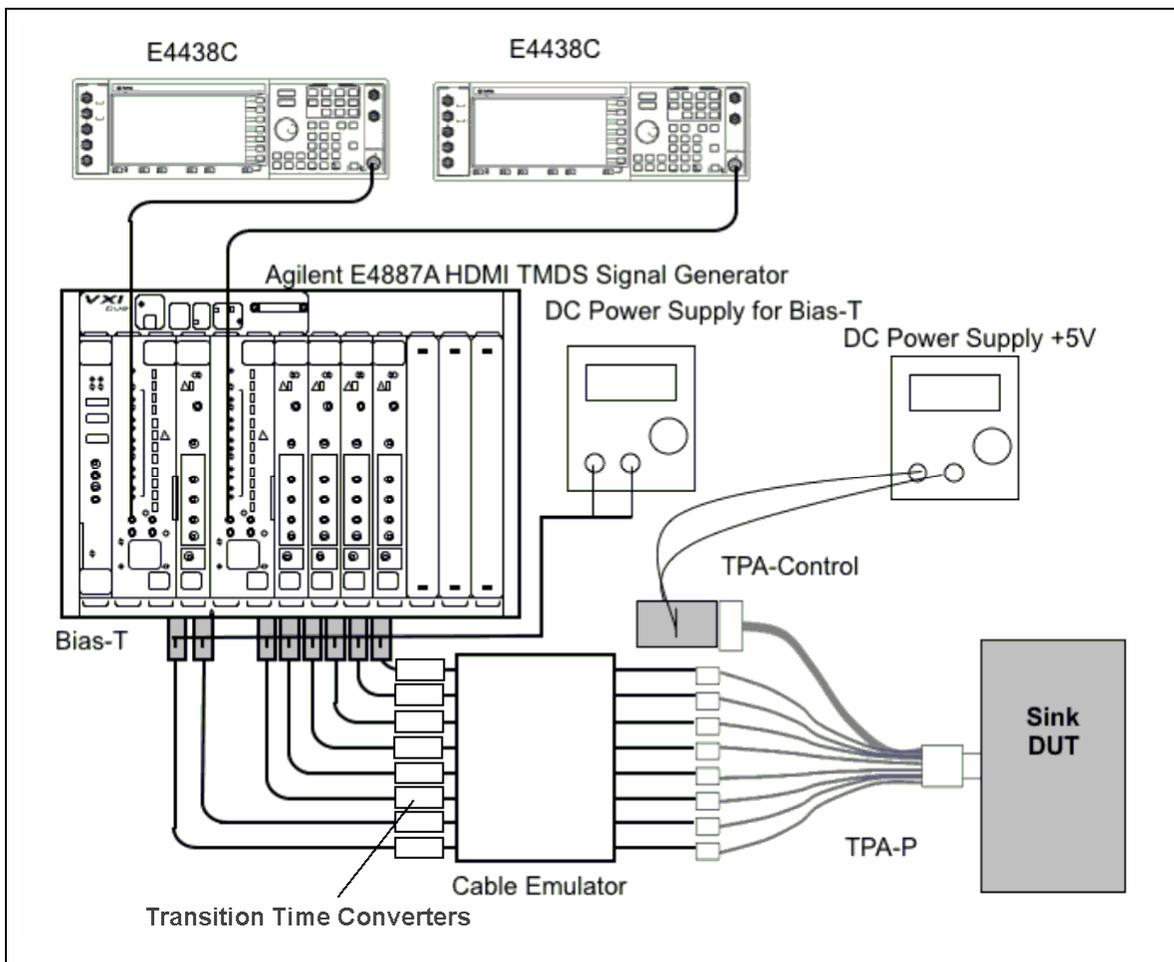
*Setup 44. Test ID 8-7: TMDS – Jitter Tolerance - Agilent*
