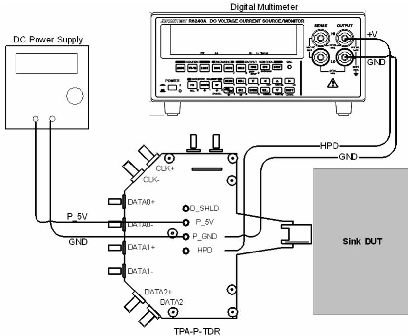
Setup 47. Test ID 8-10: HPD Output Voltage
