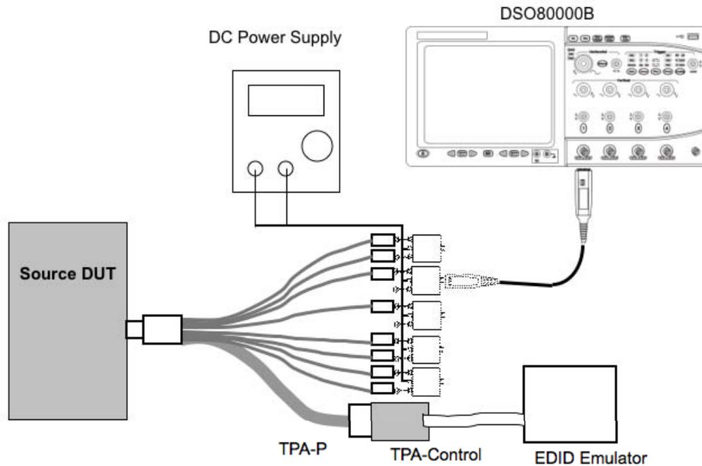
Setup 14. Test ID 7-2: TMDS –VBL: Agilent DSO80000B
