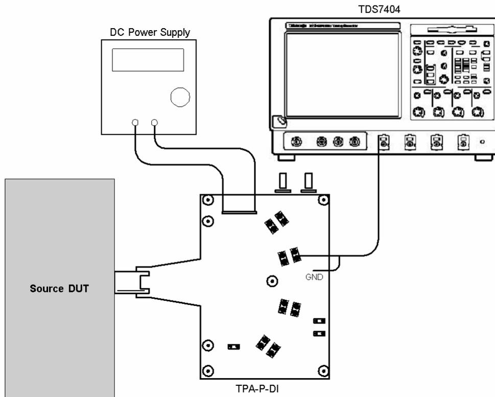
Setup 16. Test ID 7-4: TMDS – TBRISEB, TBFALLB: Tektronix TDS7404
