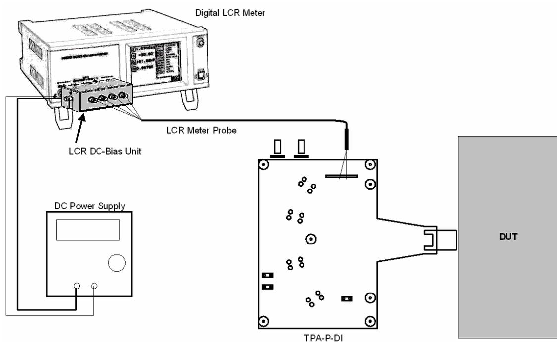
Setup 46. Test ID 8-9: DDC/CEC Line Capacitance and Voltage
