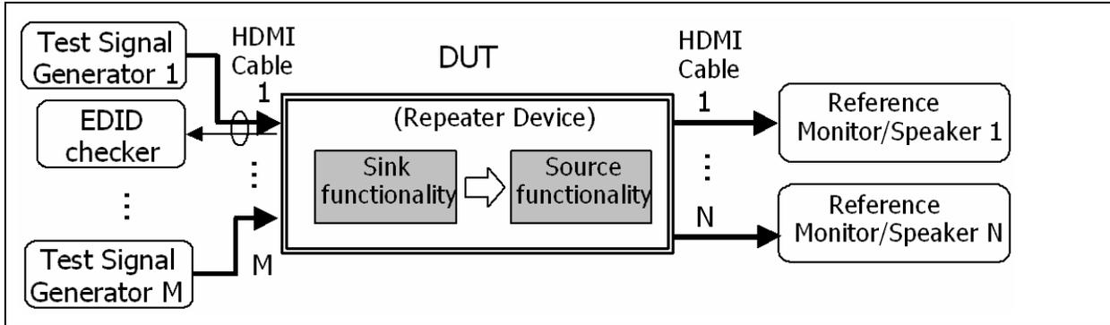
Figure 9-5 Testing of Sink Functionality
