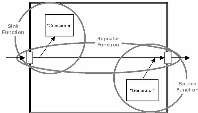
Figure 9-3 Source vs. Sink vs. Repeater Functionality
