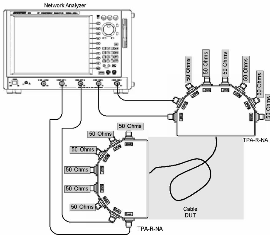
Setup 8. Test ID 5-7: Attenuation and Phase: ADVANTEST
