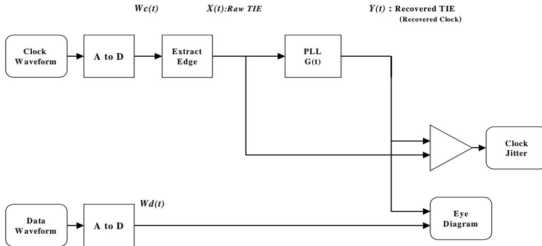
Fig.2 Conventional Clock Recovery Method
