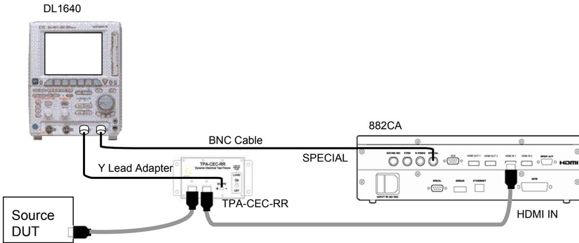
If the DUT is a sink, then instead connect the HDMI cable to the port marked "HDMI OUT 1" on the 882CA.
