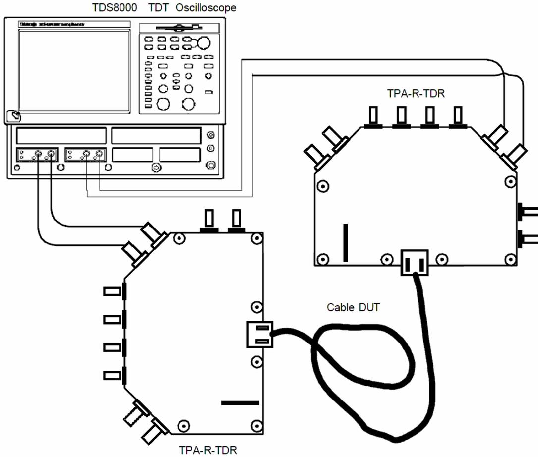
Setup 4. Test ID 5-4: Intra-Pair Skew: Tektronix
