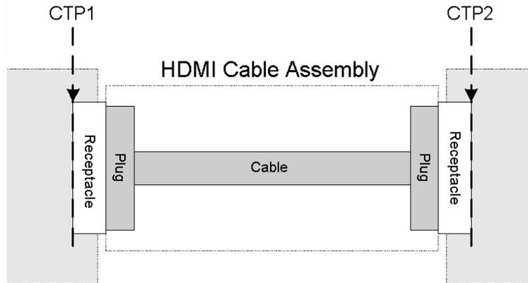
Figure 5-1 Cable Test Points
