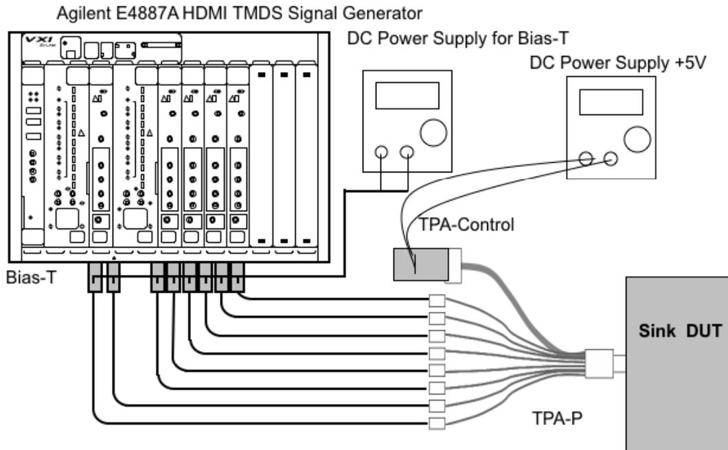
Setup 41. Test ID 8-6: TMDS – Intra-Pair Skew - Agilent
