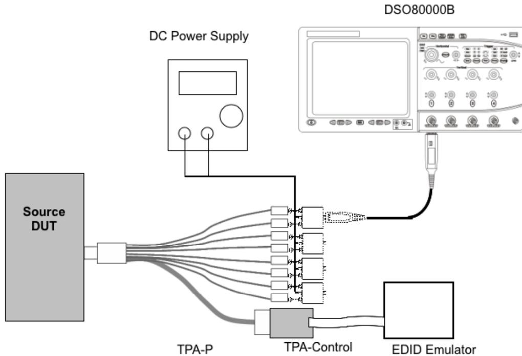
Setup 30. Test ID 7-9: TMDS – Clock Jitter - Agilent
