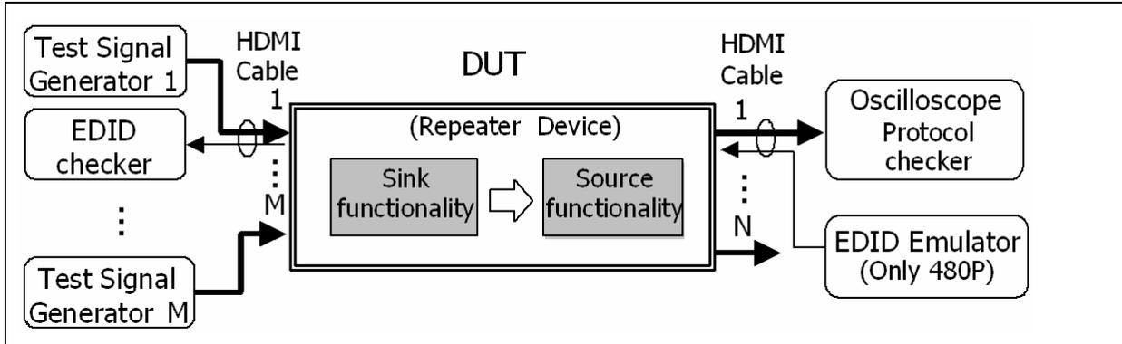
Figure 9-4 Testing of Source Functionality
