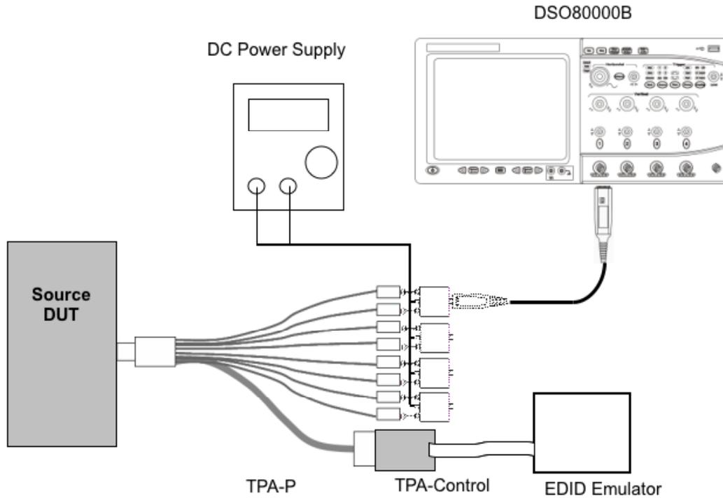
Setup 27. Test ID 7-8: TMDS – Clock Duty Cycle - Agilent
