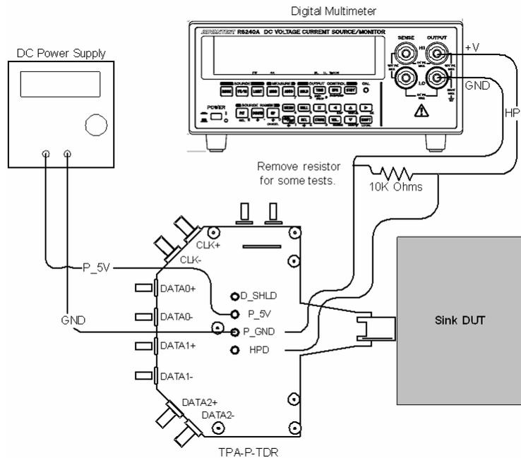
Setup 48. Test ID 8-11: HPD Output Resistance
