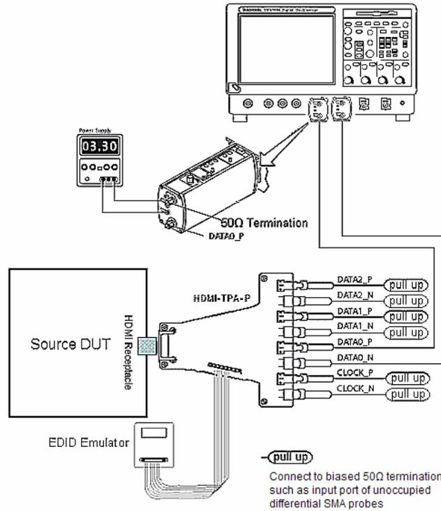
Setup 23. Test ID 7-7: TMD5 – Intra-Pair Skew - Tektronix DPO70804
