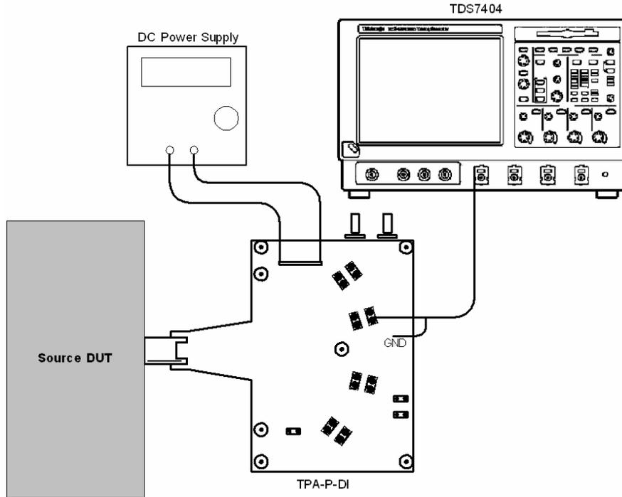
Setup 25. Test ID 7-8: TMDS – Clock Duty Cycle - Tektronix TDS7404
