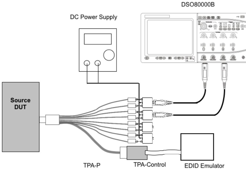
Setup 33. Test ID 7-10: TMDS – Data Eye Diagram - Agilent
