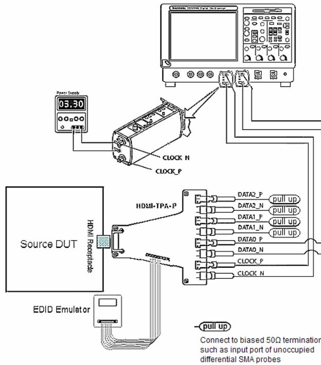
Setup 17. Test ID 7-4: TMDS – TBRISEB, TBFALLB: Tektronix DPO70804
