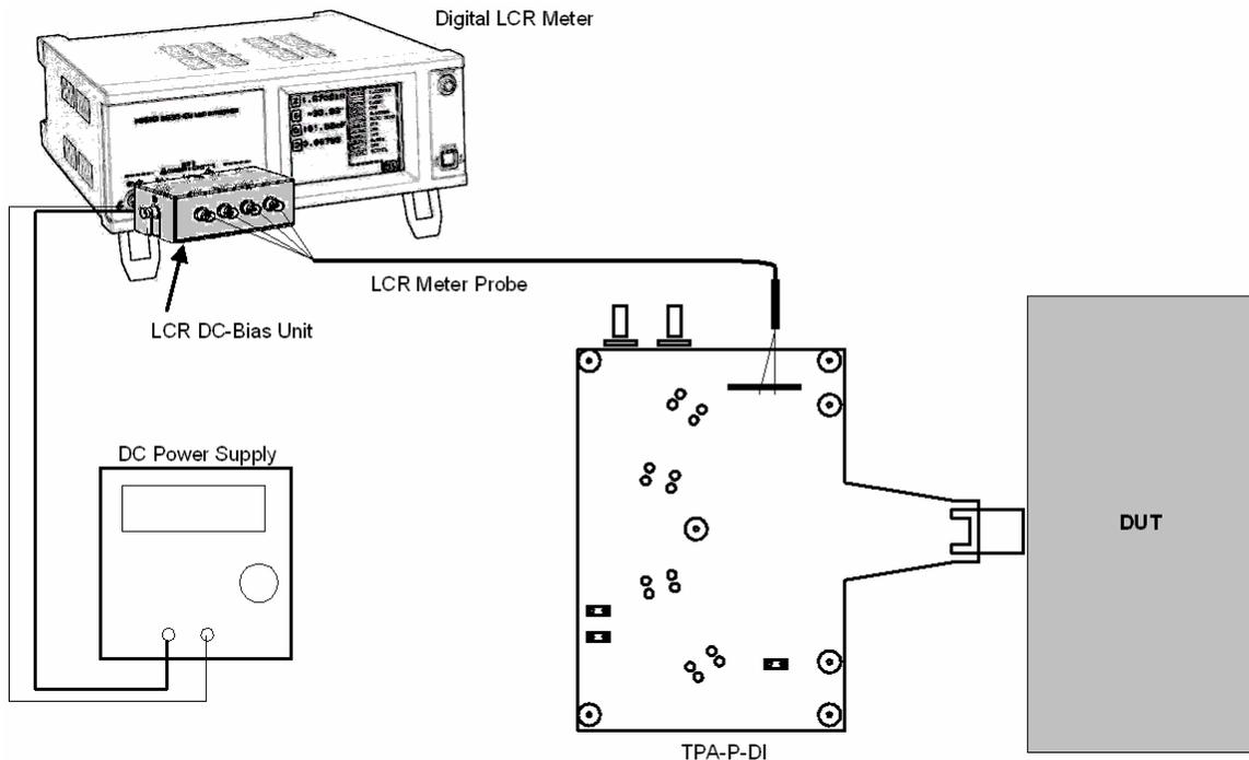
Setup 36. Test ID 7-13: DDC/CEC Capacitance and Voltage
