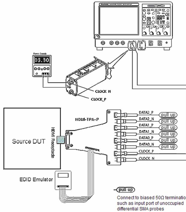
Setup 26. Test ID 7-8: TMDS – Clock Duty Cycle - Tektronix DPO70804
