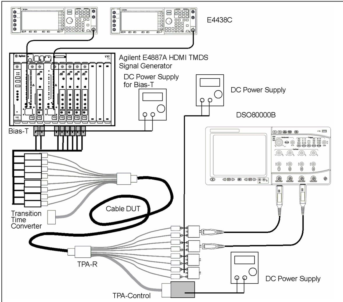
Setup 3. Test ID 5-3: TMDS Data Eye Diagram: Agilent ParBERT-based Setup
