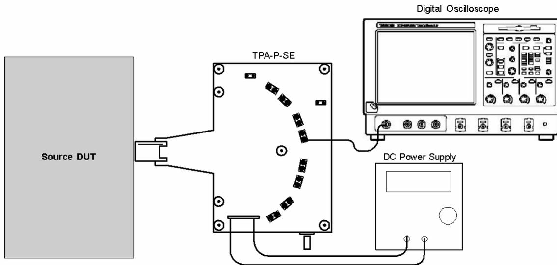
Setup 12. Test ID 7-2: TMDS –VBL: Tektronix TDS7404
