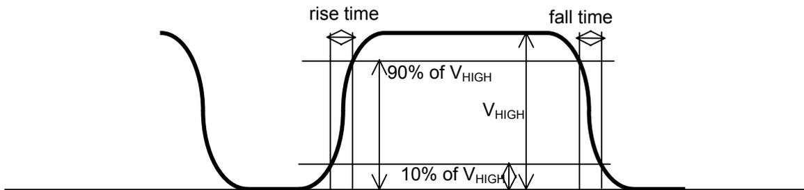
CECT Figure 5 Rise Time and Fall Time in CEC waveform
