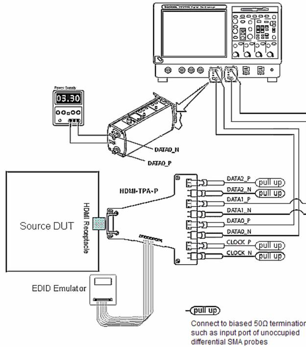
Setup 20. Test ID 7-6: TMDS – Inter-Pair Skew - Tektronix DPO70804
