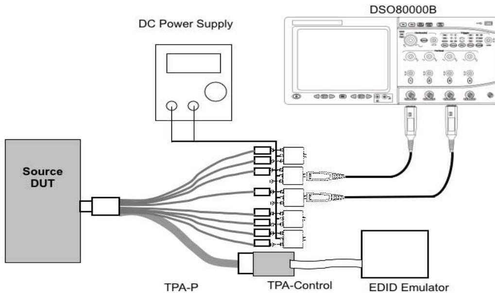
Setup 24. Test ID 7-7: TMDS – Intra-Pair Skew - Agilent
