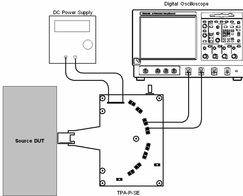
Setup 22. Test ID 7-7: TMDS – Intra-Pair Skew - Tektronix TDS7404
