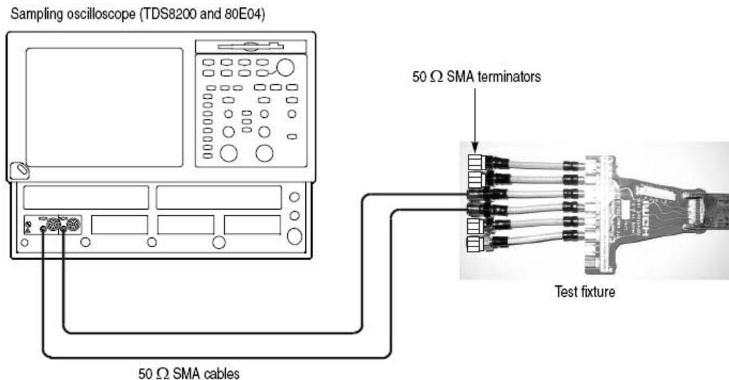
Setup 45. Test ID 8-8: TMDS – Differential Impedance
