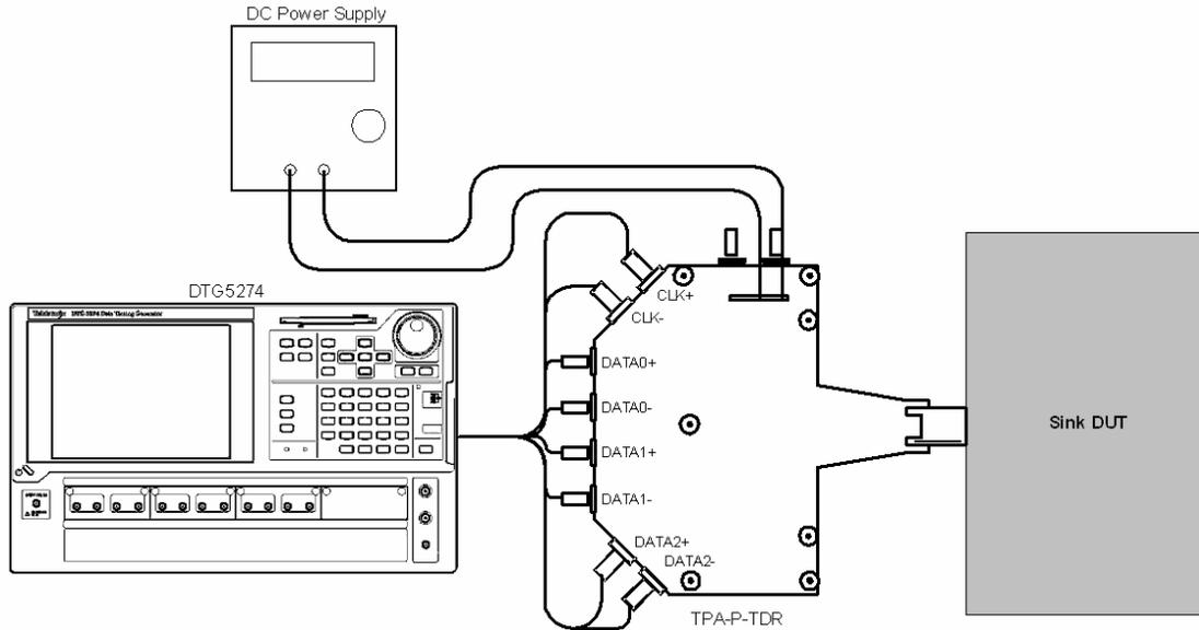
Setup 40. Test ID 8-6: TMDS – Intra-Pair Skew
