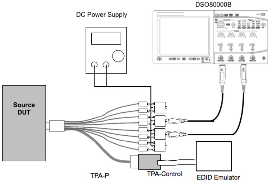
Setup 21. Test ID 7-6: TMDS – Inter-Pair Skew – Agilent DSO80000B
