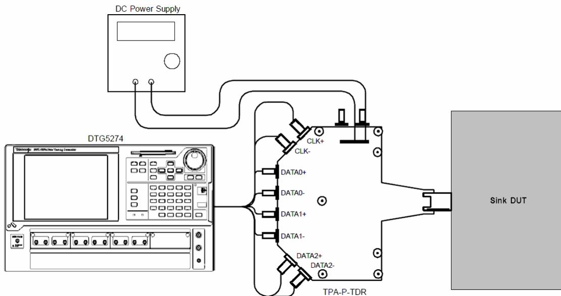
Setup 38. Test ID 8-5: TMDS – Min/Max Differential Swing Tolerance – Tektronix
