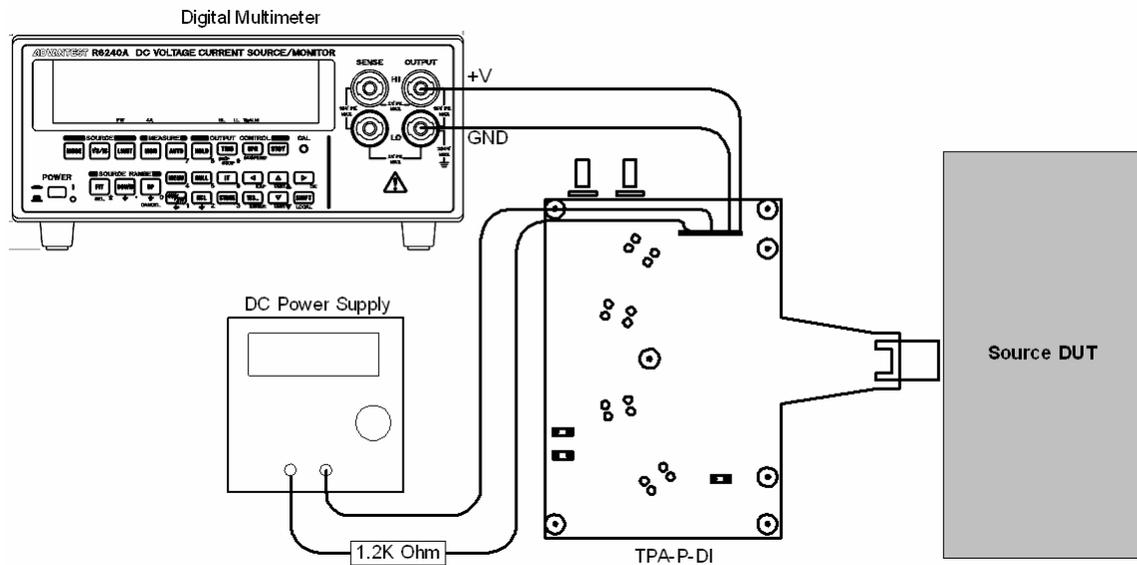
Setup 35. Test ID 7-12: Hot Plug Detect
