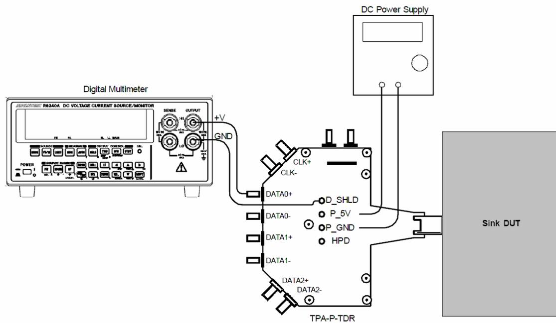
Setup 37. Test ID 8-4: TMDS – Termination Voltage
