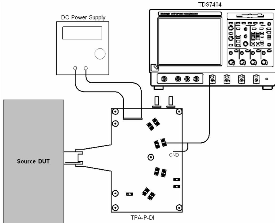
Setup 28. Test ID 7-9: TMDs – Clock Jitter - Tektronix TDS7404
