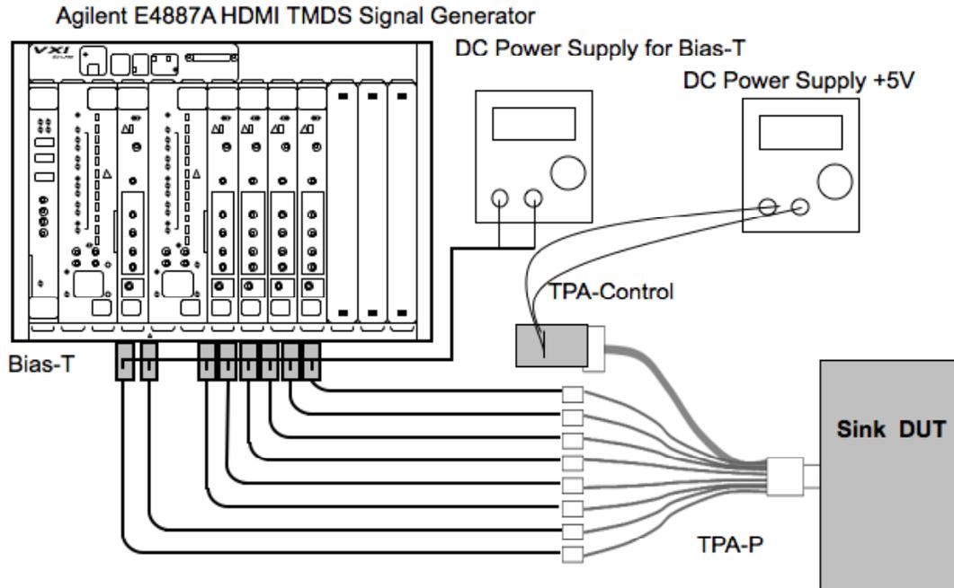
Setup 39. Test ID 8-5: TMDS – Min/Max Differential Swing Tolerance - Agilent
