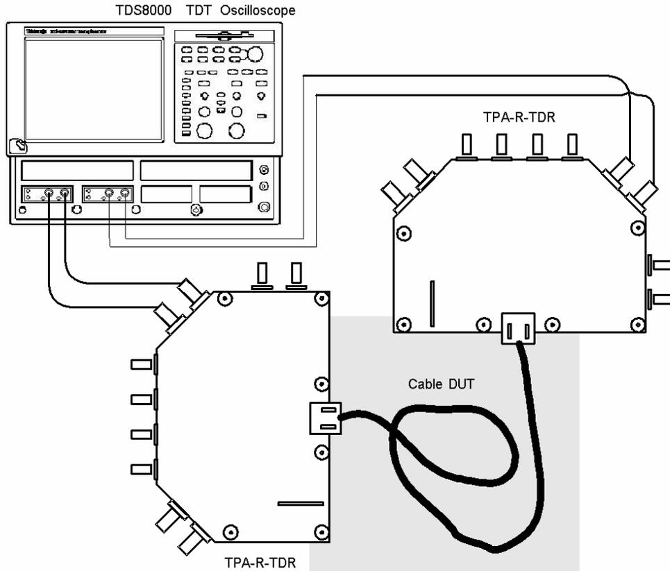
Setup 5. Test ID 5-5: Inter-Pair Skew: Tektronix
