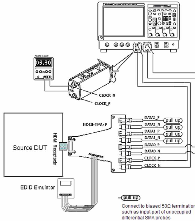
Setup 29. Test ID 7-9: TMDs – Clock Jitter - Tektronix DPO70804
