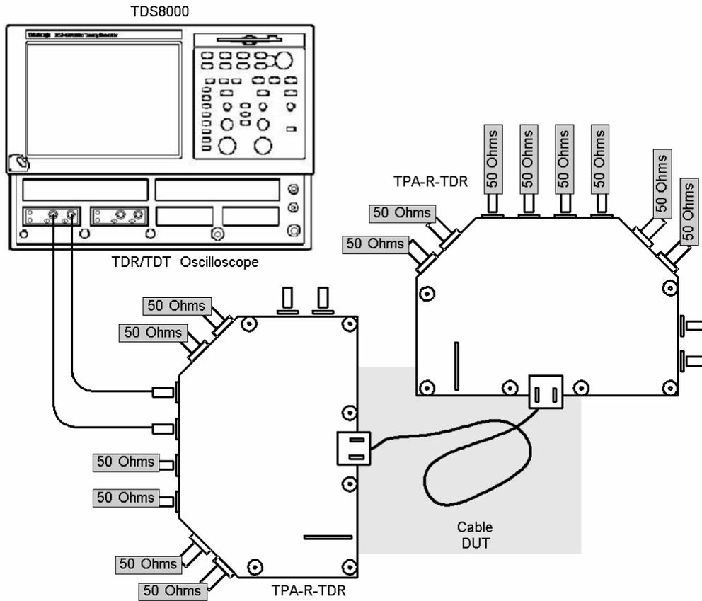
Setup 10. Test ID 5-8: Differential Impedance: Tektronix
