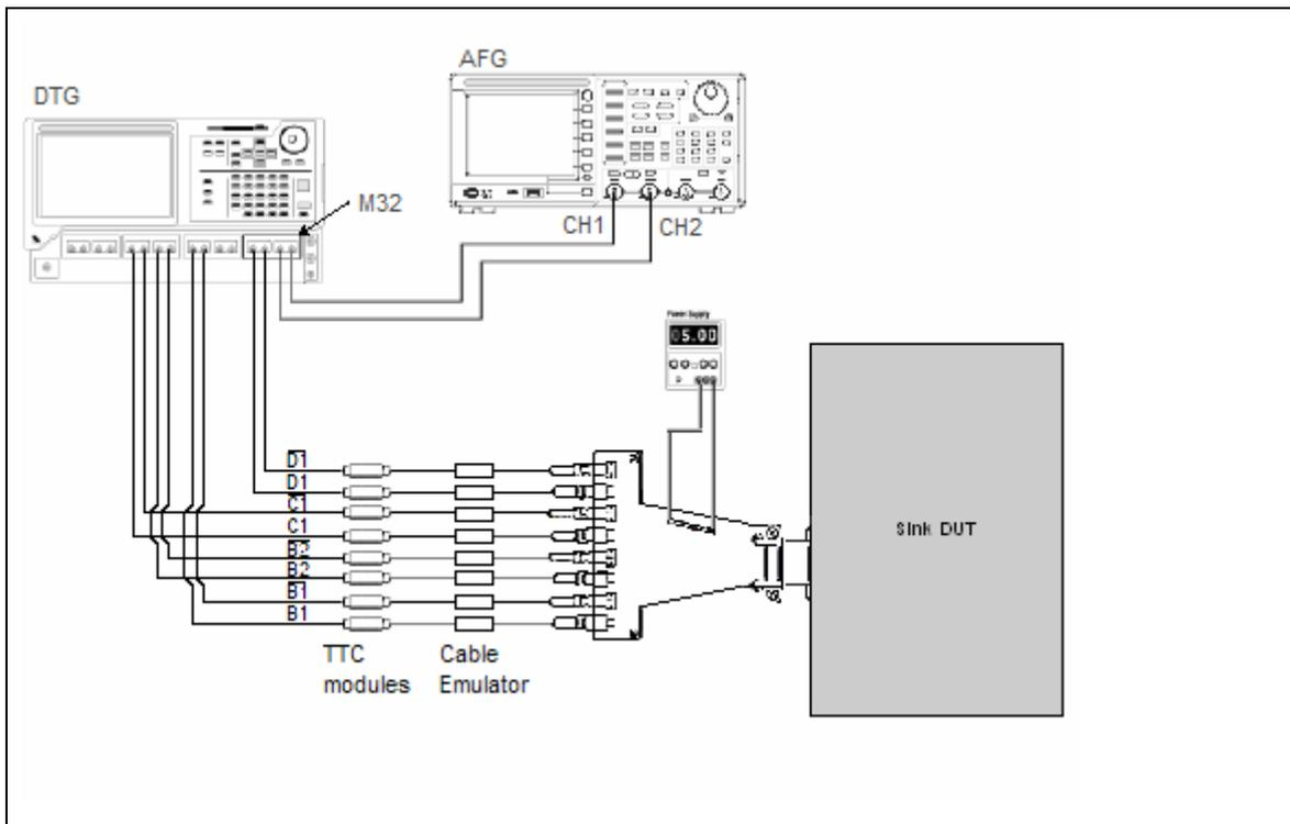
Setup 43. Test ID 8-7: TMDS – Jitter Tolerance: Tektronix All Frequencies
