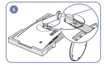
On the back of the monitor, align and push the COVER REAR SUB in the groove in the direction of the arrow.
