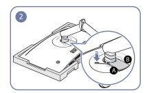
Insert the dedicated disassembly pin into tabs (A) Remove the and (B), then use the pin as a lever to lift the COVER direction.
