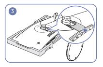
Remove the COVER REAR SUB in the arrow direction.
