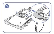
Remove the COVER REAR TOP in the direction of the arrow.
