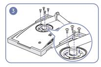
Use the screws on the stand to tightly fasten.
