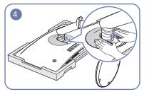
On the back of the monitor, use your fingers to lift the COVER REAR TOP in the direction of the arrows, as shown in the image.
